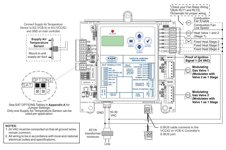
Figure 13: Communications Wiring - Two Modulating Valves, One Ignitor, One Stage
