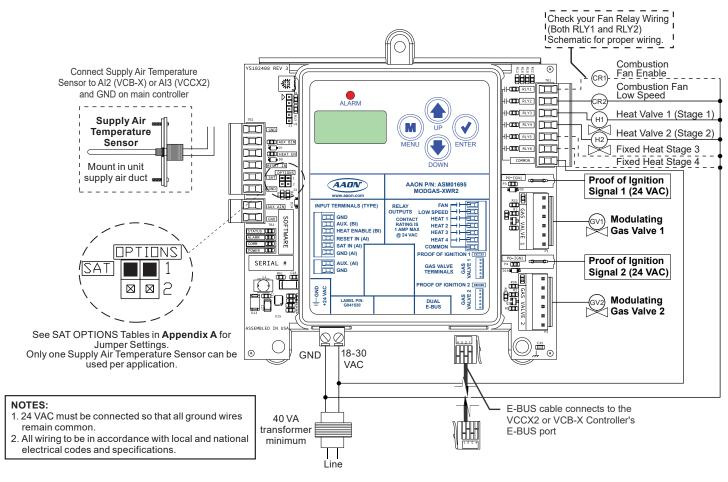
Figure 11: Communications Wiring - Two Modulating Valves, Two Ignitors, Two Stages
