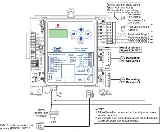
Figure 6: Stand-Alone Wiring - Secondary Board 2V1IGN1S
