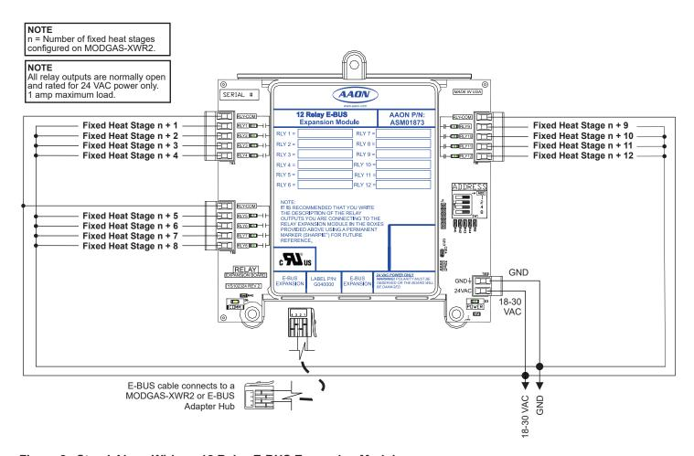
Figure 8: Stand-Alone Wiring - 12 Relay E-BUS Expansion Module
