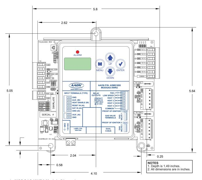
Figure 1: MODGAS-XWR2 Module Dimensions
