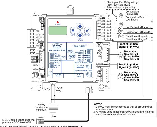
Figure 4: Stand-Alone Wiring - Secondary Board 2V2IGN2S
