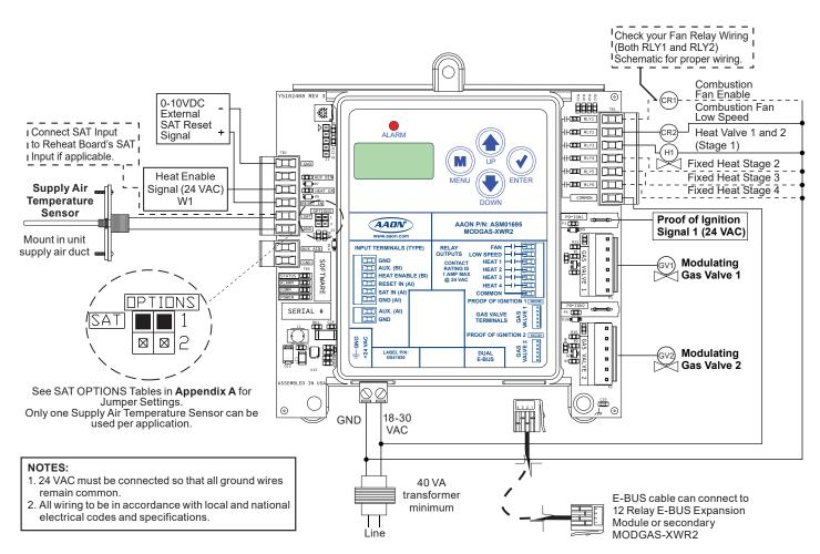
Figure 5: Stand-Alone Wiring - Two Modulating Valves, One Ignitor, One Stage
