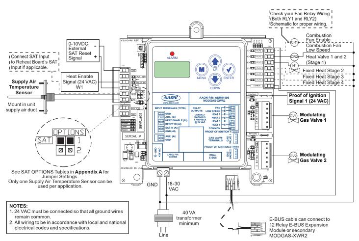
Figure 7: Stand-Alone Wiring - Two Modulating Valves, Two Ignitors, One Stage
