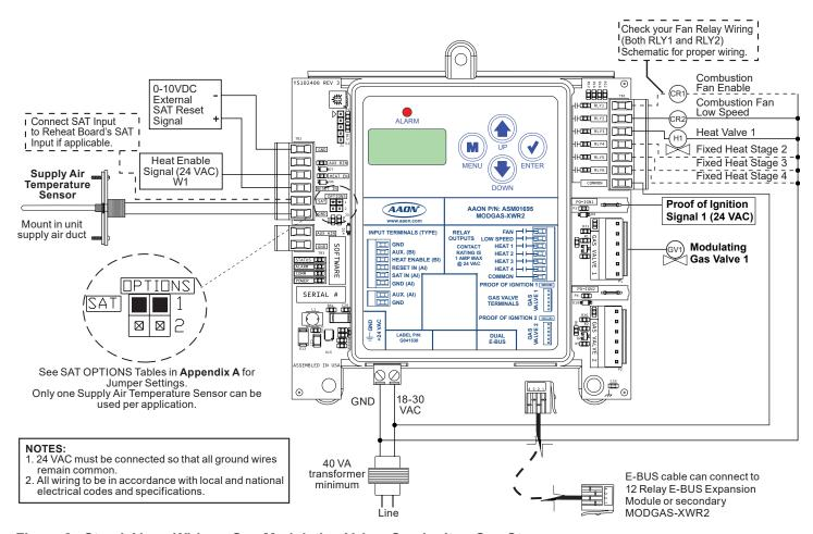
Figure 2: Stand-Alone Wiring - One Modulating Valve, One Ignitor, One Stage
