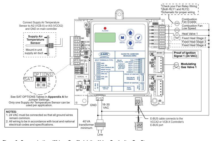
Figure 9: Communications Wiring - One Modulating Valve, One Ignitor, One Stage
