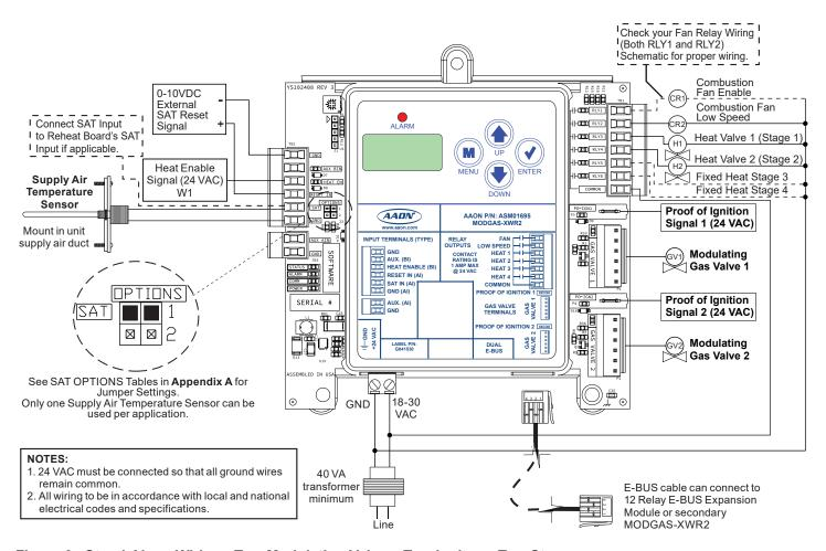
Figure 3: Stand-Alone Wiring - Two Modulating Valves, Two Ignitors, Two Stages
