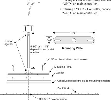
Figure 17: Supply Air Temperature Sensor Installation
