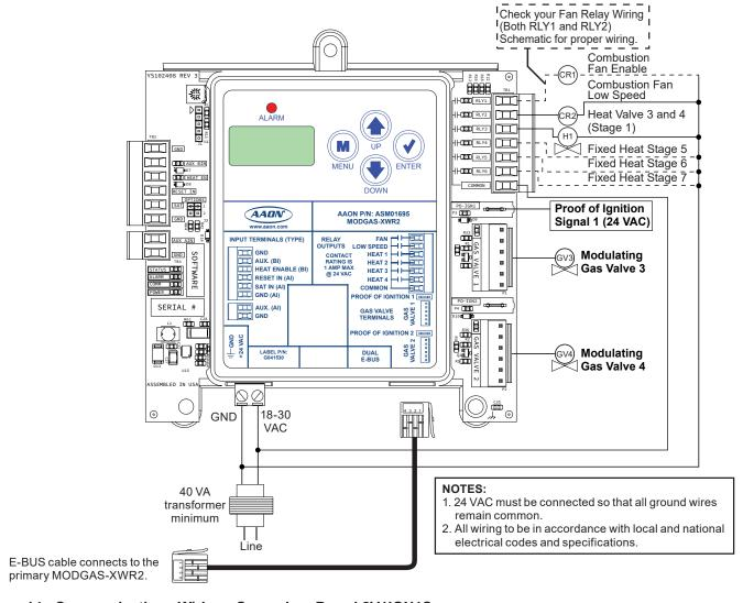
Figure 14: Communications Wiring - Secondary Board 2V1IGN1S
