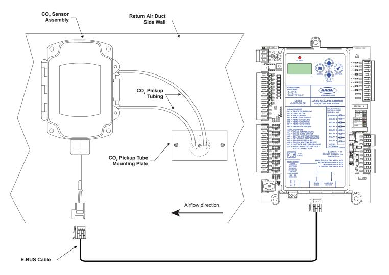
Figure 2: Duct-Mounted E-BUS CO, Sensor Wiring and Components
