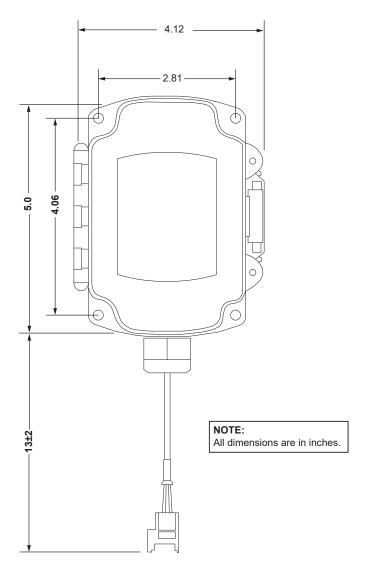
Figure 1: Duct-Mounted E-BUS CO<sub>2</sub> Sensor Dimensions
