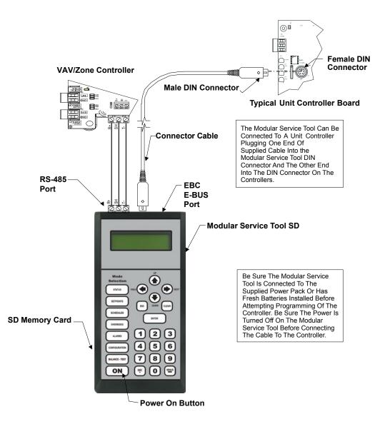
Figure 2: Modular Service Tool SD
