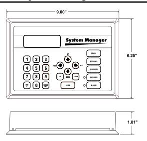
Figure 3: Modular System Manager SD Dimensions
