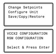
On the first screen, scroll down to the 'Configure Unit' option and *press* **<ENTER>**. On the second screen, *select* VCCX2 Configuration and then press **<ENTER>**. This will take you to the first Configuration Screen shown below.
