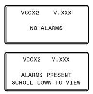
*Press*  $< \square >$  to scroll through all the alarms for the controller that the Modular Service Tool is connected to.
