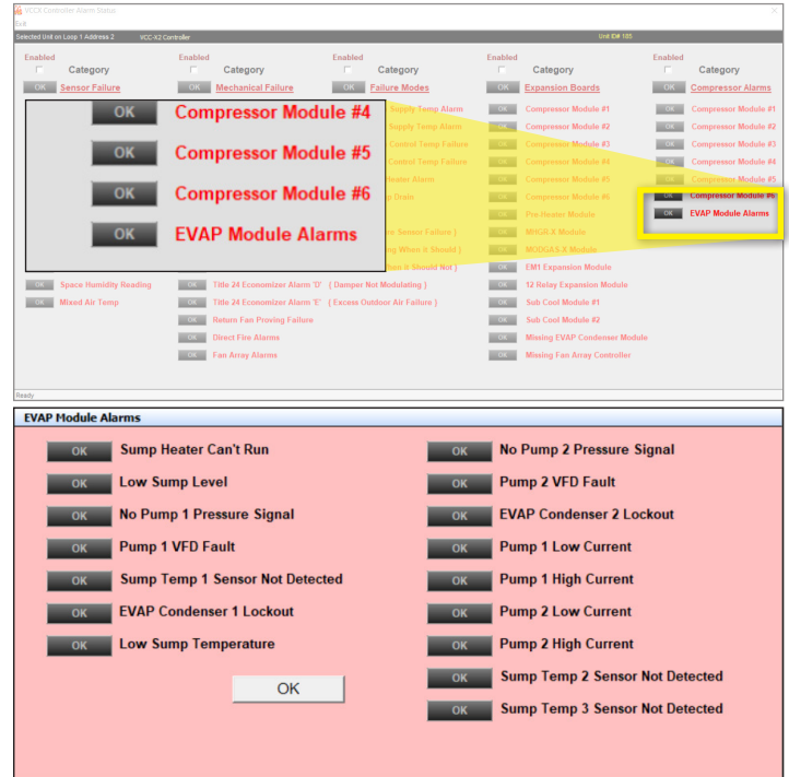
Figure 18: Prism 2 EVAP Module Alarms Screen
