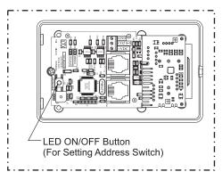
View of Back Side of Sensor Cover & Circuit Board (With Sensor Base Removed)
