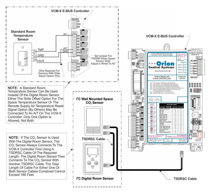
Figure 2: Wall Mounted Space CO. Sensor & Digital Room Sensor Wiring for VCM-X E-BUS Controller
