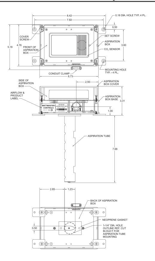
Figure 5: Mounting and Cable Installation for Duct-Mounted CO<sub>2</sub> Sensor
