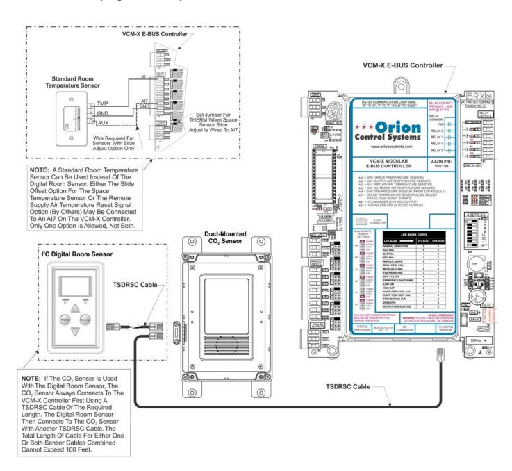
Figure 3: Duct-Mounted CO<sub>2</sub> Sensor & Digital Room Sensor Wiring for VCM-X E-BUS Controller
