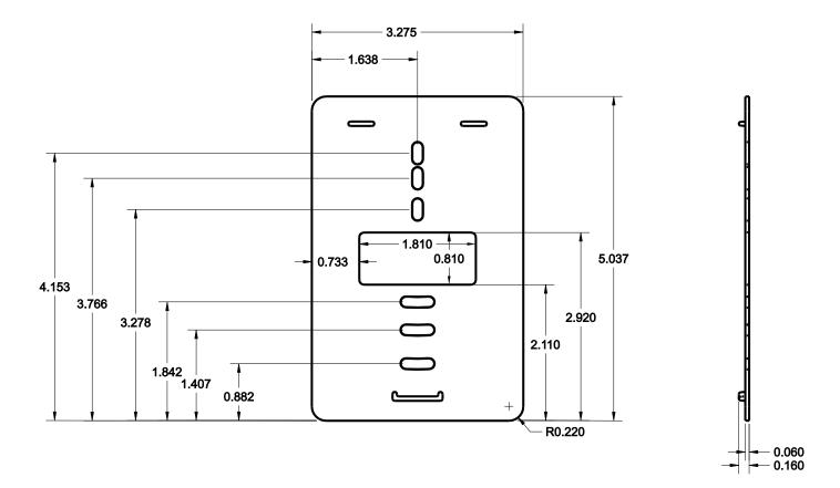
**Figure 8: Mounting Plate Dimensions**
