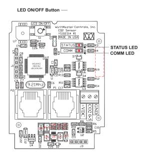
Figure 6: LED ON/OFF Button and Board LEDs
