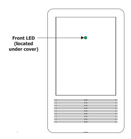
Figure 7: CO<sub>2</sub> Sensor's Front LED
