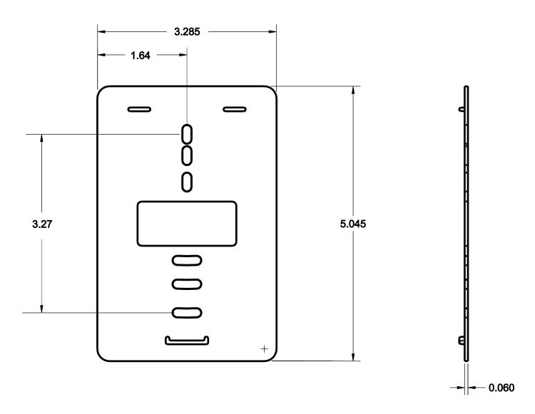
**Figure 6: Mounting Plate Dimensions**
