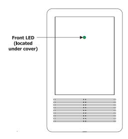
Figure 5: Wall Mounted E-BUS CO<sub>2</sub> Sensor's Front
