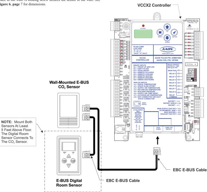
Figure 2: Wall Mounted Space E-BUS CO Sensor & E-BUS Digital Room Sensor Wiring for VCCX2 Controller
