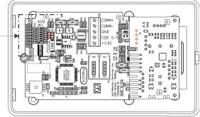
E-BUS CO, Sensor with Back Cover Removed
