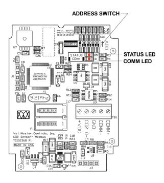
Figure 4: Address Switch and Board LEDs
