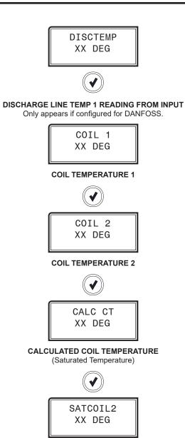
**SATURATION LINE: TEMP 2 READING FROM INPUT** Only appears if configured for two compressors/circuits.
