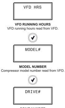
DRIVE NUMBER Type of Danfoss VFD - CDS803 or CDS303.
