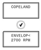
MINIMUM COMPRESSOR SPEED LIMIT Minimum compressor envelope speed in rpm.
