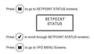
**Note:** There are three separate VFD menus. The one that appears is dependent on your unit's configuration.
