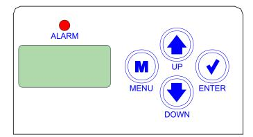
Figure 8: LCD Display and Navigation Keys
