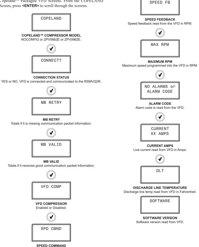
Commanded speed in RPM.
