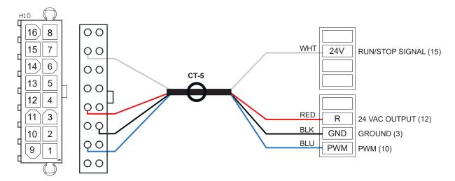
Figure 1-8: H10 WSHP Harness Wiring
