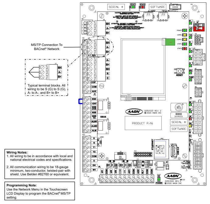
Figure 1-14: BACnet® Legacy Connection to MS/TP BAS Network
