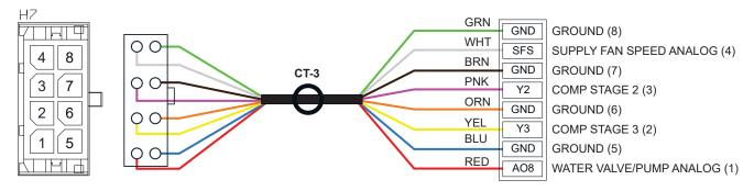
Figure 1-6: H7 Variable Capacity Harness Wiring
