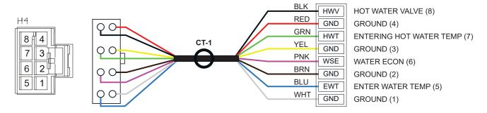
Figure 1-4: H4 Water Harness Wiring
