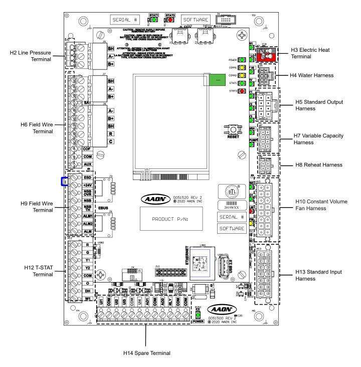
Figure 1-2: Pioneer Gold Controller Terminal and Harness Components
