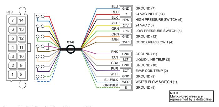
Figure 1-9: H13 Standard Input Harness Wiring
