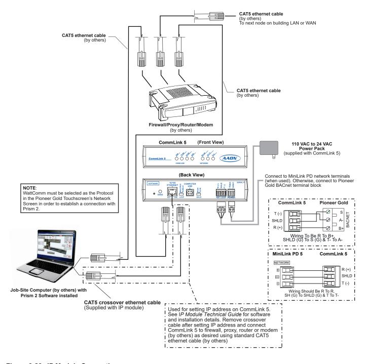
Figure 3-23: IP Module Connection
