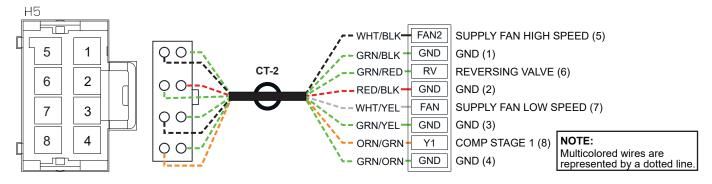
Figure 1-5: H5 Standard Output Harness Wiring
