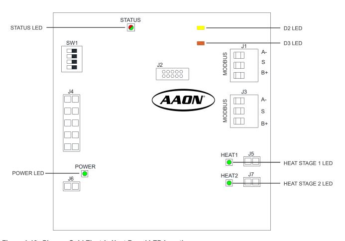
Figure 1-13: Pioneer Gold Electric Heat Board LED Locations
