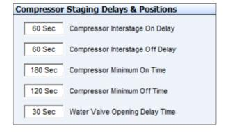
Figure 3-7: Compressor Staging Delays & Positions Screen
