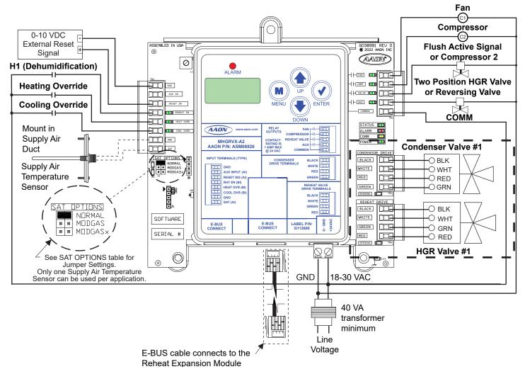
Figure 3: MHGRVX-A2 Stand-Alone Wiring
