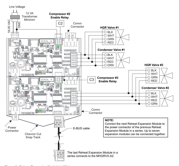
Figure 8: Reheat Expansion Module(s) Wiring
