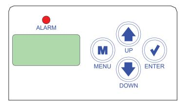
Figure 4: LCD Display and Navigation Keys
