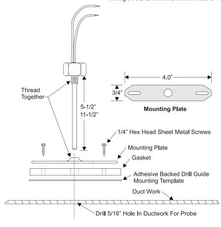
Figure 6: Supply Air Temperature Sensor Installation
