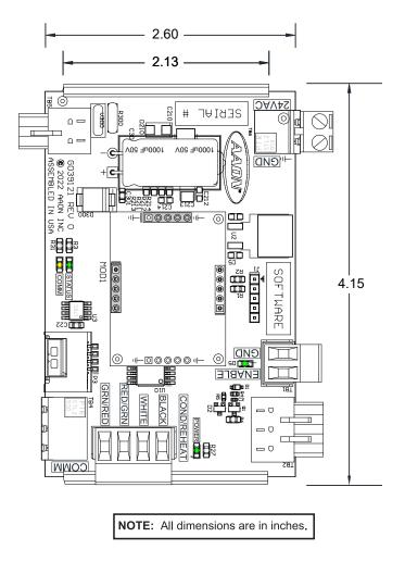
Figure 7: Reheat Expansion Module Dimensions
