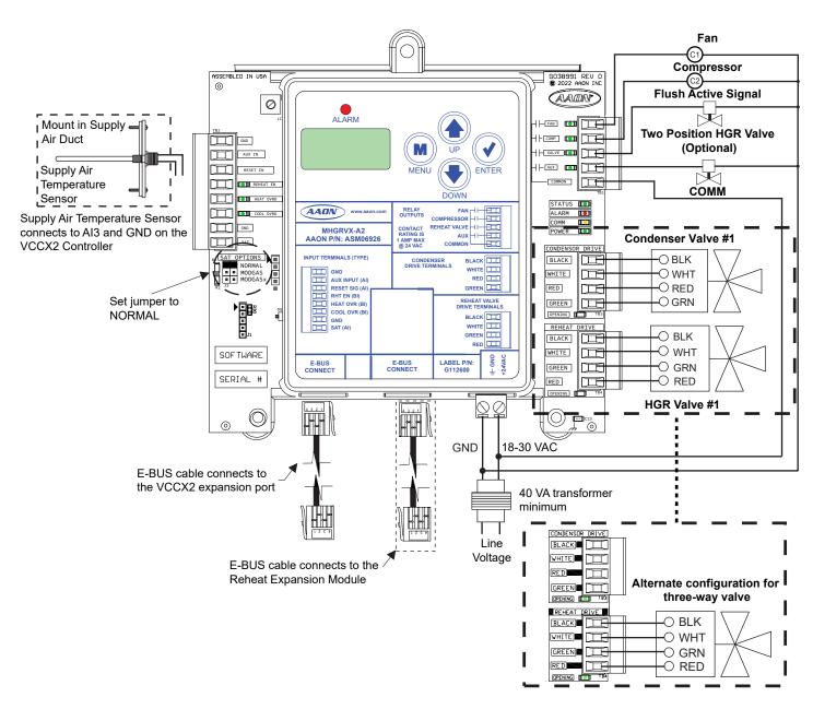
Figure 2: MHGRVX-A2 to AAON Unit Controller Wiring
