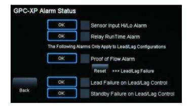
Figure 35: GPC-XP Controller Alarm Status Screen
