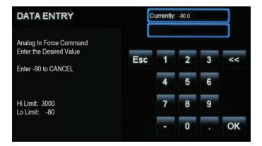
Figure 17: Sensor Override Data Entry Screen
