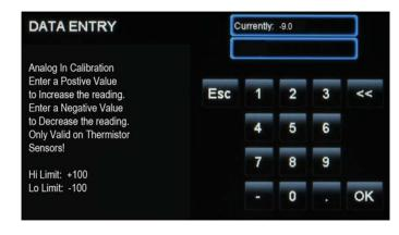
Figure 16: Calibrate Sensor Data Entry Screen
