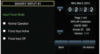
Figure 19: Binary Input Force Mode Screen
