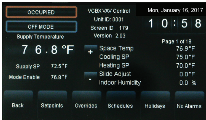
Figure 18: VCC-X/VCB-X Controller Status Screen 1
