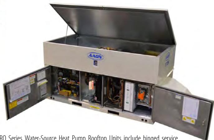
RQ Series Water-Source Heat Pump Rooftop Units include hinged service access doors to all airside components, compressor, controls, and waterside components. Coaxial refrigerant-to-water heat exchanger and waterside components are in a rigid polyurethane foam insulated service compartment.
