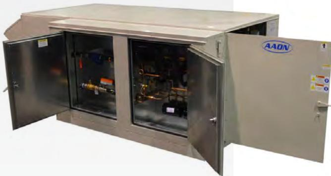
RN Series Water-Source Heat Pump Rooftop Units include brazed plate refrigerant-to-water heat exchanger and waterside components in a rigid polyurethane foam insulated service compartment. Heat pump refrigeration components are also accessible from this compartment.
