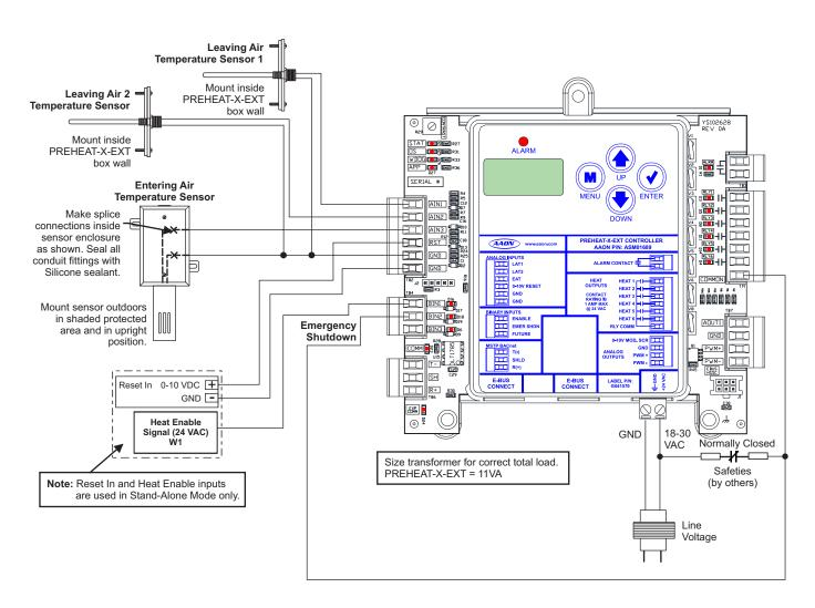
Figure 2: PREHEAT-X-EXT Inputs Wiring Diagram
