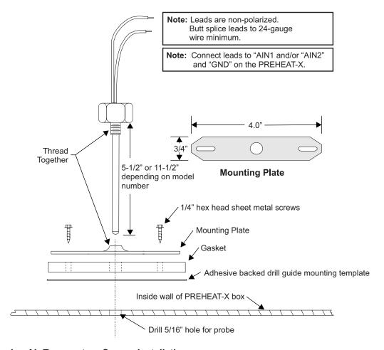
Figure 7: Leaving Air Temperature Sensor Installation
