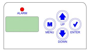
Figure 4: LCD Display and Navigation Keys
