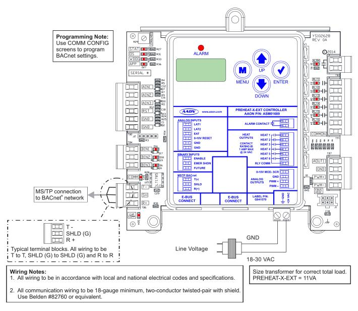
Figure 8: PREHEAT-X-EXT BACnet Connection to MS/TP Network
