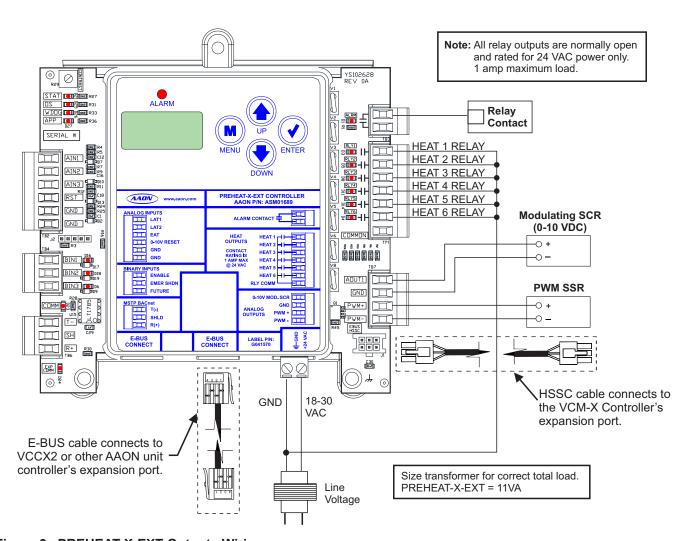
Figure 3: PREHEAT-X-EXT Outputs Wiring
